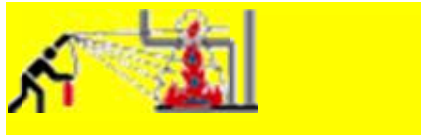
liquid fires and fires caused by dripping substances should be extinguished from the top down
